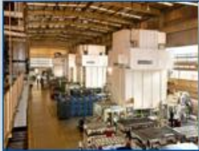
3 Cold Transfer Presses (2x 1.600 Tn & 1x 2.000Tn)
